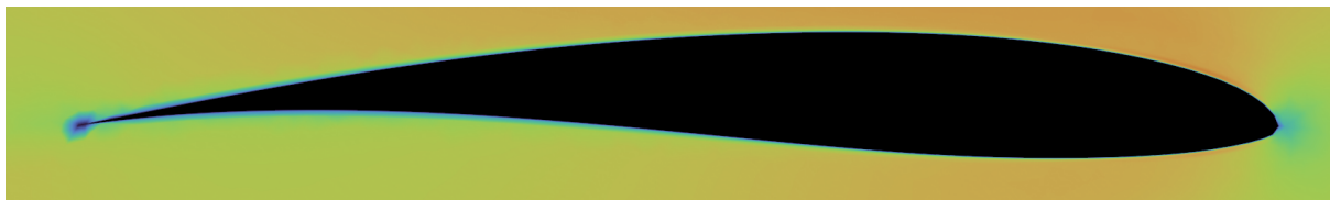
Figure 11: Representation of the velocity distribution around one airfoil section, at 50 cm from the wing root. The zone in green/blue around the airfoil represents the boundary layer, very thin in this simulation. In general, the aim is to obtain this kind of streamflow for a wide range of flight conditions, in order to ensure that the wing airfoil works always at optimal conditions.
