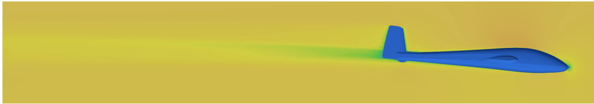
Figure 10: Velocity distribution around the model. It is possible to note clearly the zone at slightly higher speed on top of the canopy (color orange/red) and the low-velocity wake behind the model (color green(light yellow)). It is important to evaluate the velocity distribution around the fuselage, to ensure that the streamflow remains adherent to the model surface in every part of the fuselage itself. In addition, the shape and the velocity distribution inside the wake provide an indication of the overall drag of the fuselage and of the entire model.
